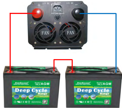
24VDC Inverter Connection
