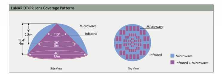
Complies with EN 50131-1, Grade 2, Class II FCC Part 15 applies for RK150T VdS applies for RK2000S
